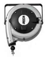
The Rotolift is equipped with a cable stop device and enables a steel cable to be wound up, from which objects that are only lowered onto the work surface while they are in use can be suspended. After use, these objects can be lifted up beyond the working area by releasing the locking device. The steel cable (ø 3 mm) is encased in a transparent nylon sheath ø 6 mm.
